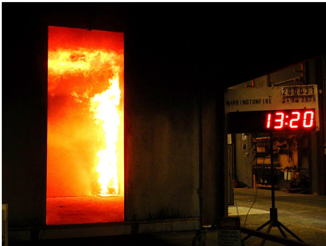
Figure 16 The system 03 minutes and 20 seconds after the burner output was increased to 300 kW.
