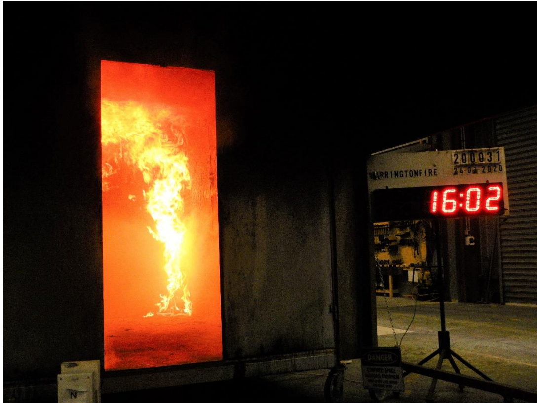
Figure 17 The system 06 minutes and 02 seconds after the burner output was increased to 300 kW.
