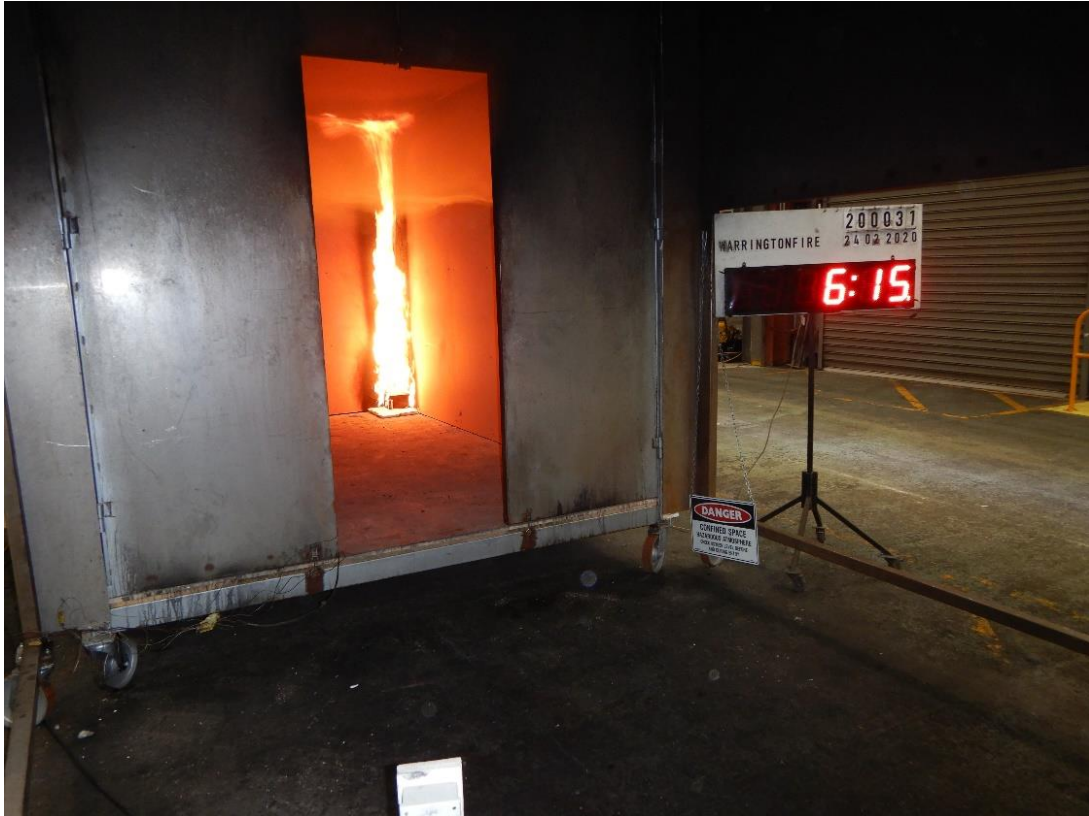
Figure 13 The system 06 minutes and 15 seconds after burner ignition with the burner output of 100 kW.
