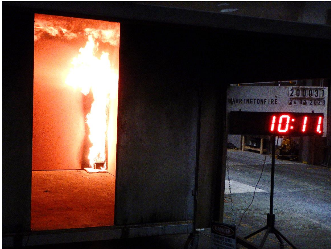
Figure 15 The system 11 seconds after the burner output was increased to 300 kW.
