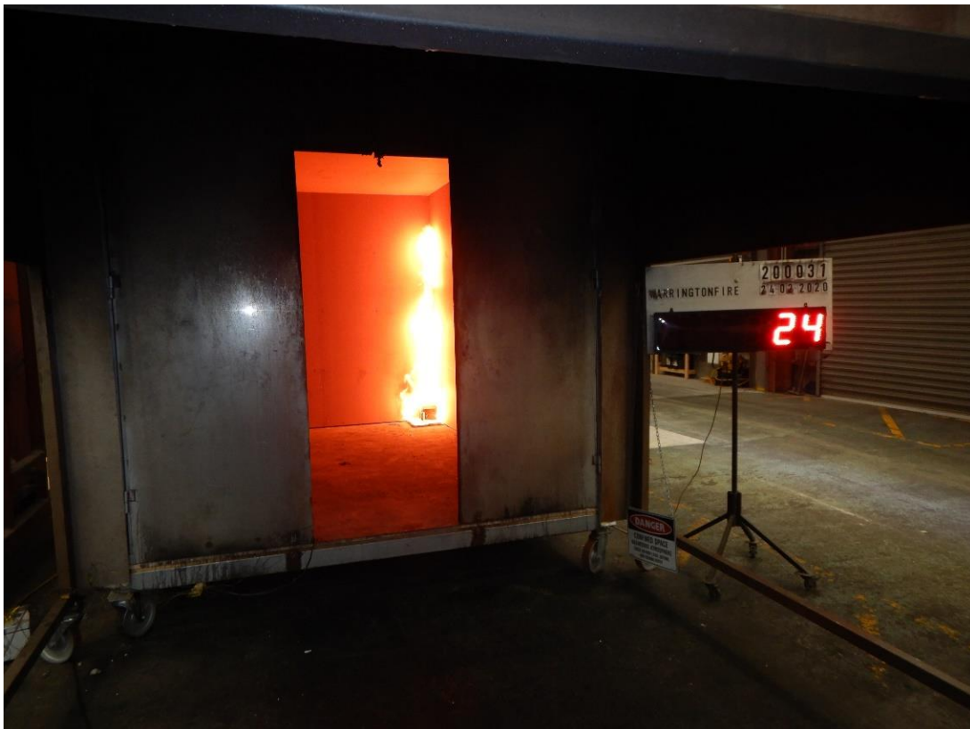
Figure 12 The system 24 seconds after burner ignition with the burner output of 100 kW.
