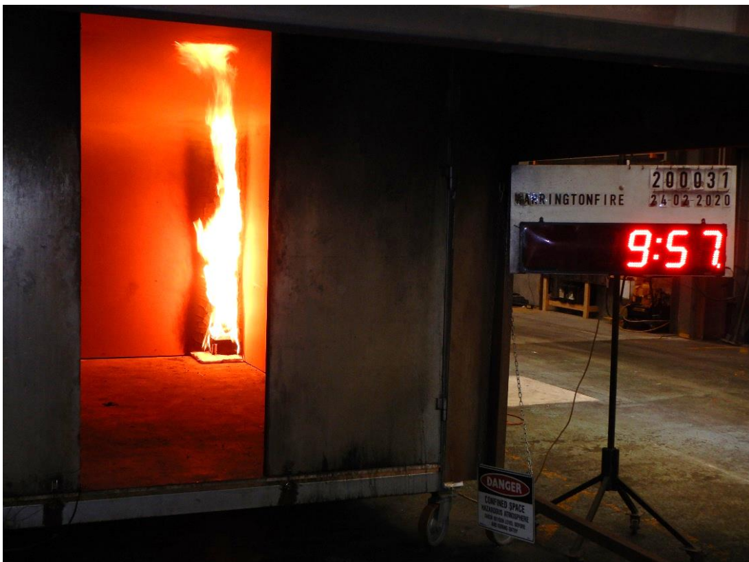
Figure 14 The system 09 minutes and 57 seconds after burner ignition with the burner output of 100 kW.
