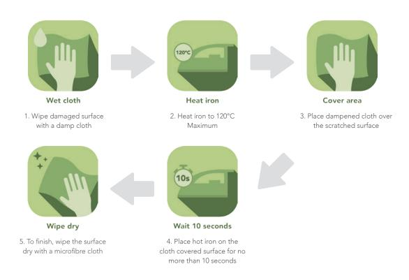
During this process, steam and heat facilitates the recovery of the CleanTouch surface. Ensure the cloth covering the damaged area is damp and creating steam. Keep the iron in constant motion and remove the iron before all moisture has left the cloth. Please note, this repair method is suitable for scratches that have not penetrated the surface layer of the laminate.
